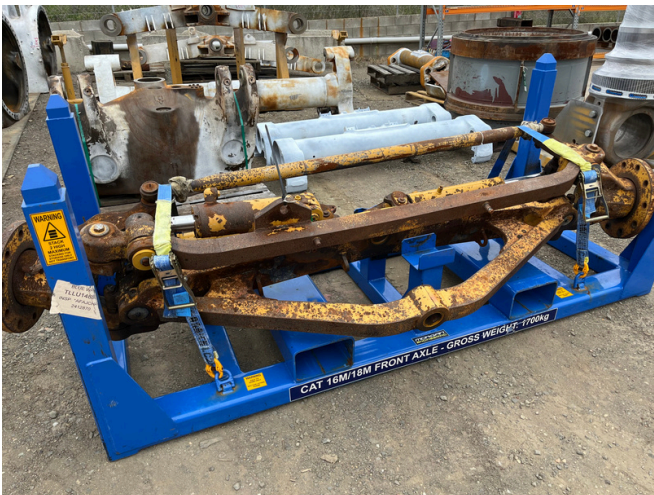
Before and after of a repaired 16M Front Axle
